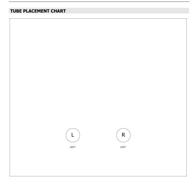
Every individually boxed tube (2) is labeled to match the above diagram. Insert each tube in the correct position.
