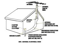
other power sources as this could be fatal. Because of the hazards involved, antenna installation should be left to a professional.
